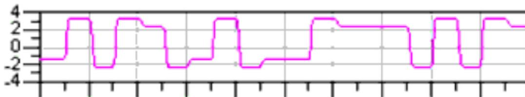
**Figure 3: This is an example of a Link Training Tx waveform corresponding to preset P03 with 2.5dB of pre-emphasis.**
