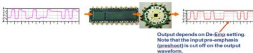
**Linear ReDriver** – Reproduces the input signal – output matches the input
