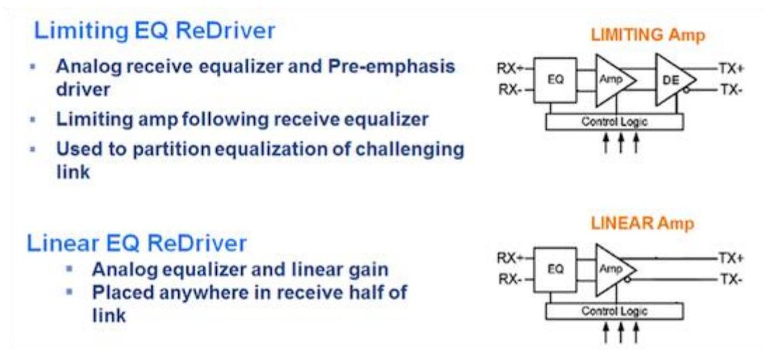
**Figure 6: The block diagram difference between regular (limiting) redrivers and linear redrivers. The final analog stage makes all the difference when PCI Express Link Training is required. (Courtesy: Pericom Semiconductor.)**
