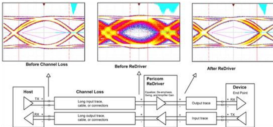
**Figure 1: Redrivers amplify and shape high frequency signals to compensate for channel “challenges.”**
