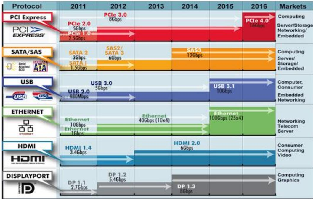
**Figure 2: Serial communications standards just keep getting faster. Along with signal integrity challenges also come specification compliance issues such as PCI Express Link Training. (Courtesy: Pericom Semiconductor.)**
