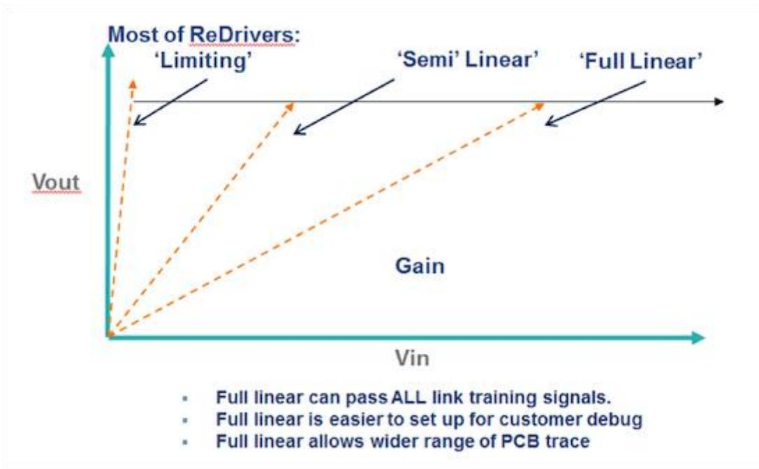
**Figure 4: The difference between linear and regular (non-linear) redrivers. Non-linear redrivers compensate for signal integrity problems, but regenerate signals that may not pass PCI Express 3.0 Link Training waveforms.**
