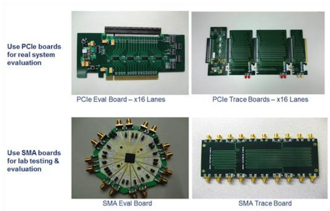
**Figure 7: Examples of linear redriver and PCI Express evaluation boards. (Courtesy: Pericom Semiconductor.)**
